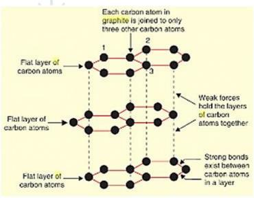
Structure of graphite (The black balls represent carbon atoms)
